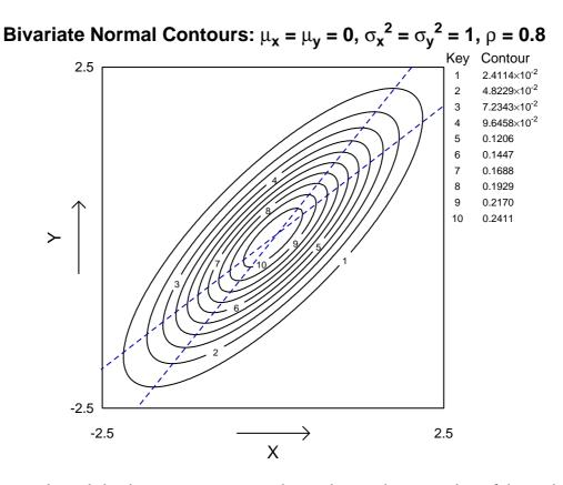
This diagram also includes the two mean regression lines indicating the mean values of the conditional distributions as functions of their arguments. These lines show the limiting positions that would be obtained with a swarm of random points following a bivariate normal distribution when plotting best-fit lines for Y as a function of X and X as a function of Y. The lines are
